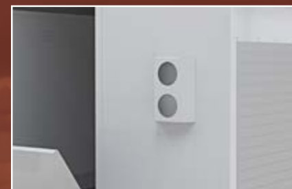
Exterior mounted light boxes to maximize space in rear compartments
