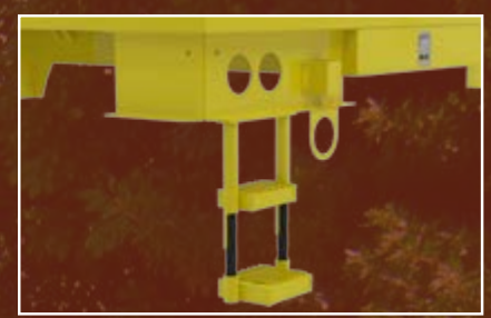
Custom strap step, strobe bracket, vise mount bracket
