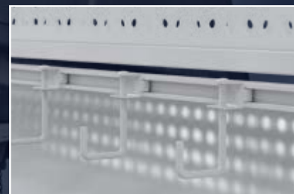
Adjustable hooks in the bed area using uni-strut rails.
