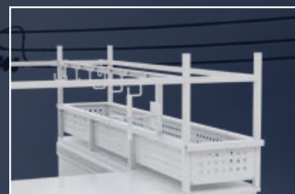
Punched metal baskets with access from bed area and the ground using "beer truck" step rail.
