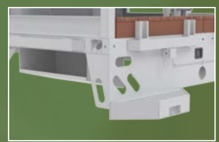
Custom rear skirt with light holes, rear steps and signholder boxes located on both sides.
