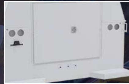
Barn style rear doors to maximize opening and bed security
