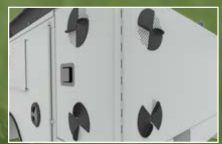
Custom rotating vents for kennel compartments
