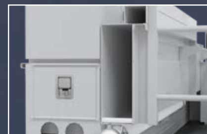
Custom vertical ladder storage
