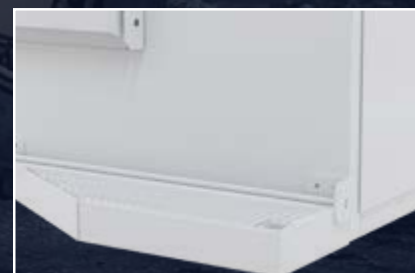
Flip up rear bumper steps allow for proper angle of departure. Also includes a vise mount.
